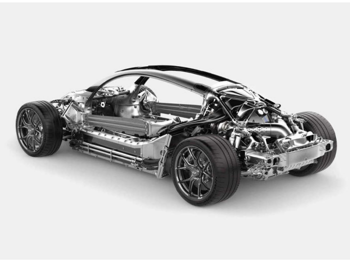
Czinger develops hybrid supercars that integrate a number of 3D printed components, including a metal chassis. Image: Czinger
